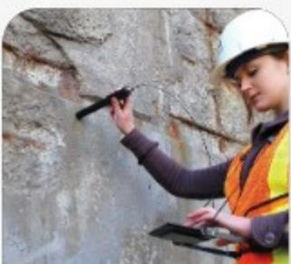
Half Cell potential testing
