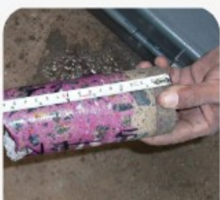
Carbonation depth measurement
