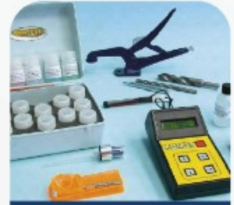
Sulphate & Chloride profile test
