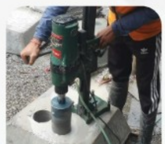
Core extraction & compression test
