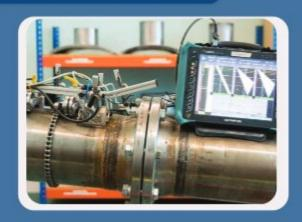
a hard wedge, a water delay line, or even inside a wheel probe, gives inspectors the ability to quickly scan large areas for corrosion, cracking, and other defects with high resolution. PAUT can be used to inspect almost any material where traditional UT methods have been utilized and is often used for weld inspections and crack detection
